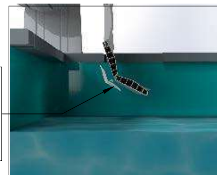
Blade guide ski: Slide the PVC ski for clipping in the female part giving the inclination of the first blade at \approx 45^\circ
