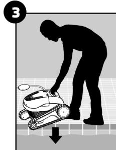
Release the Pool Cleaner and let it sink to the floor of the pool. Make sure that the floating cable is free of any obstructions.
